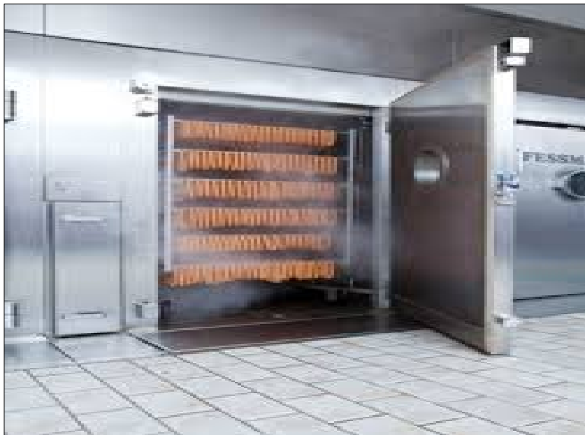
Exhibit 5. Hot dogs leaving the Industrial-Sized Smoke House
