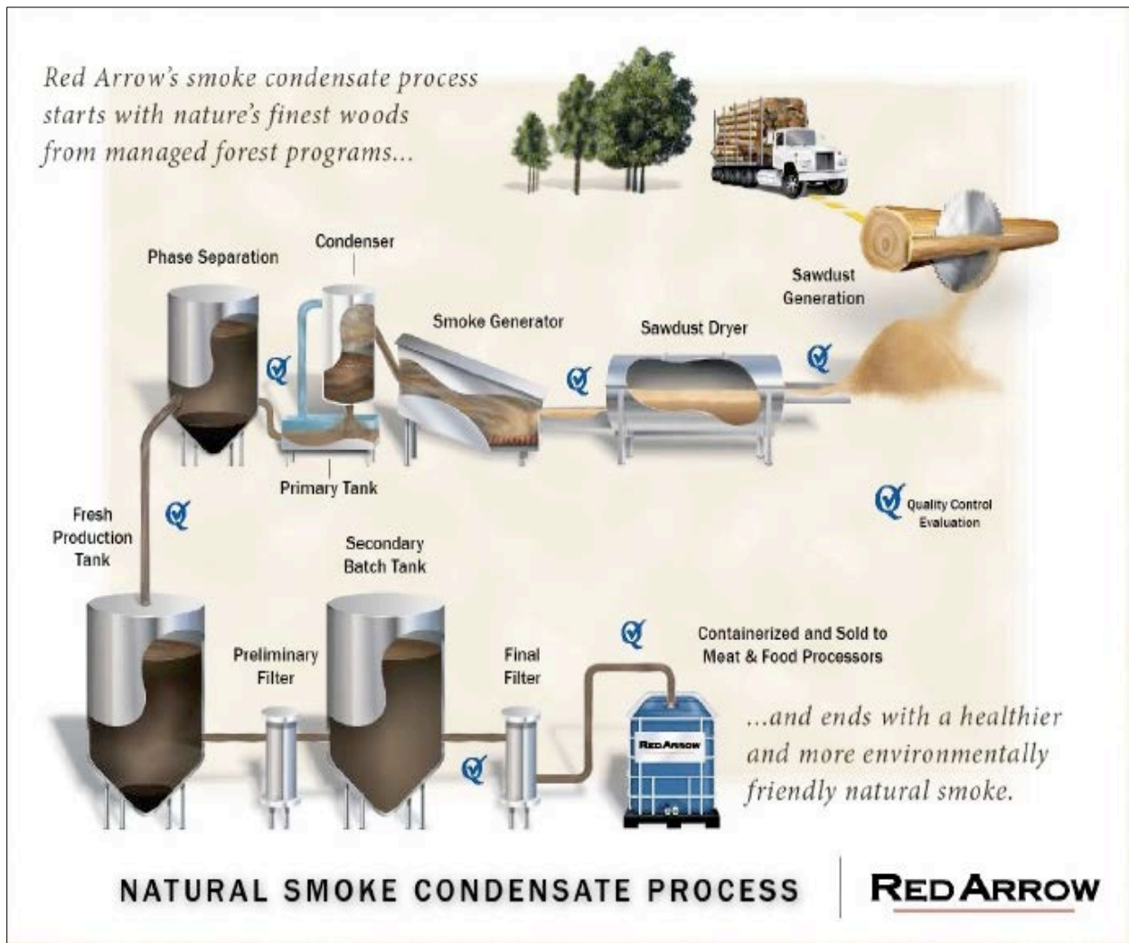
Exhibit 1. The Production of Liquid Smoke
